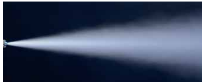
Spray pattern of a Laval nozzle
