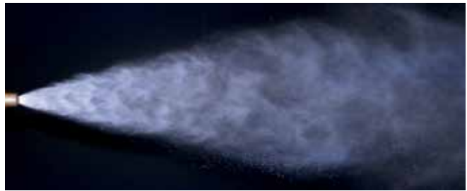
Spray pattern of the MasterNOx nozzle 30°
