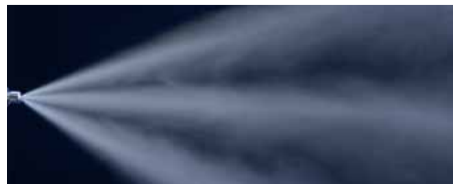
Spray pattern of the flat fan nozzle
