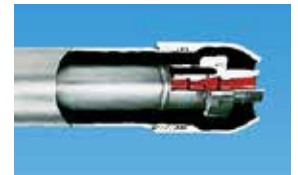
Example – Laval lance (with protective tube)
