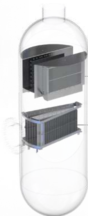
Arrangement of four mist eliminators in a pressure tank
