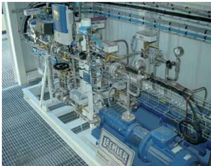
Compact pump and unit for metering in an enclosure
