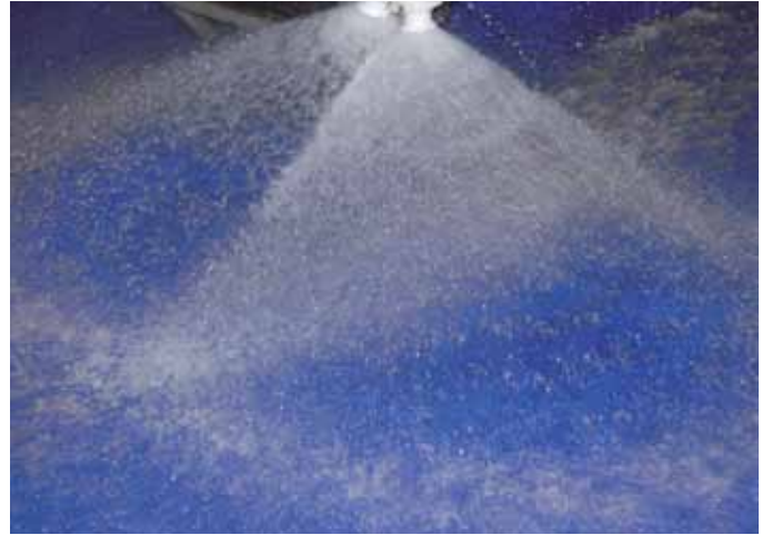
The proven equilateral Hollow Cone Nozzle TwinAbsorb®-EH generates two hollow cones by using one single supply.
