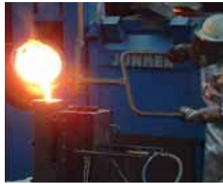
Preparation of a measurement of the nozzle heat transfer coefficient
