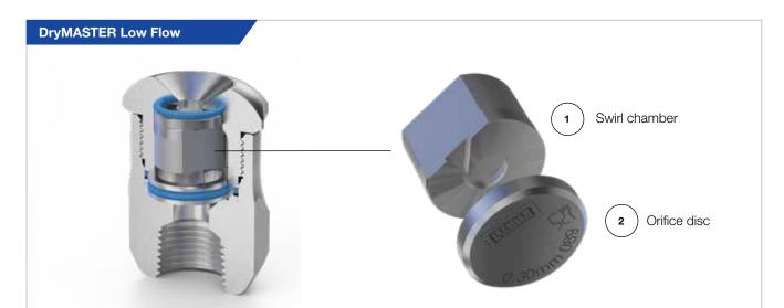
With the DryMASTER Low Flow, much smaller production volumes can be achieved with comparable back pressures and spray profiles to larger systems. The Low Flow assembly achieves this by simply swapping out the orifice disc and swirl chamber, giving the end user complete flexibility with existing plant and equipment.
