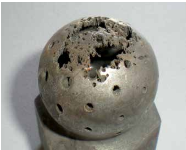
Figure 13: Chemical attack on a spray ball
