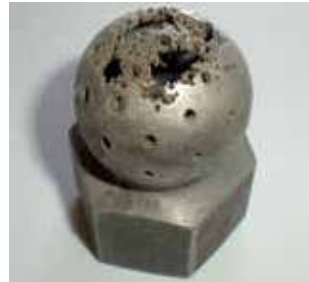
Fig. 1: Chemical corrosion of a spray ball
