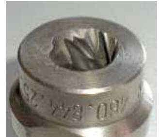
Fig. 2: Wear of a full cone nozzle
