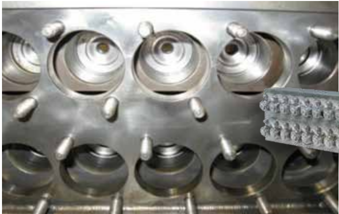
SELECTOSPRAY® header after acid cleaning
