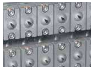
25mm valve pitch allows for a compact header design
