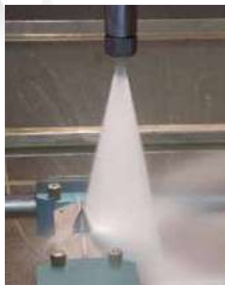
Documentation of a spray impact measurement
