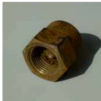
Clogged vane of a full cone nozzle
