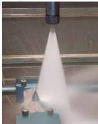
Documentation of a spray impact measurement
