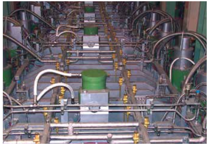
Horizontal segments with Mastercooler SMART nozzles
