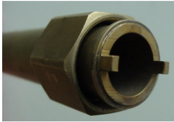
Fig. 18: Twin key alignment for tip and pipe
