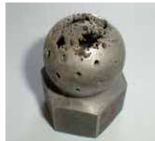
Figure 18: Chemical corrosion of a spray ball
