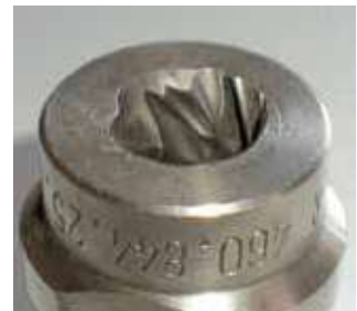
Figure 19: Wear of a full cone nozzle
