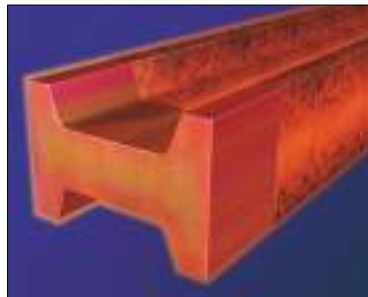
Beam partially descaled
