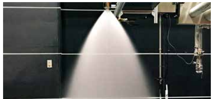
Spillback line closed (max. injection), spray angle approx. 80 – 85°
