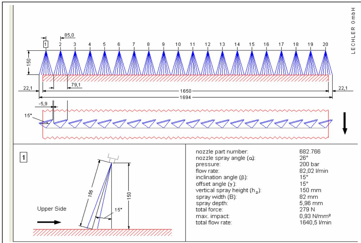
Figure 10 - Example of computer simulation with Lechler “DESCALE” program of existing situation with no overlap between adjacent sprays
