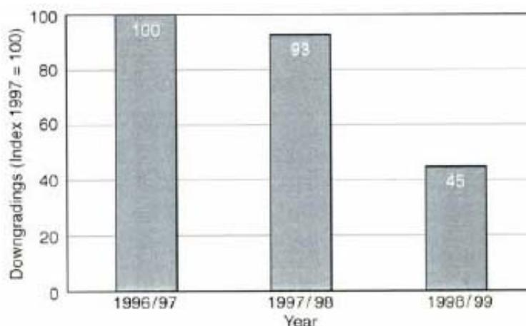
Figure 13 - Development of strip downgradings in TKS Bochum due to rolled in scale
