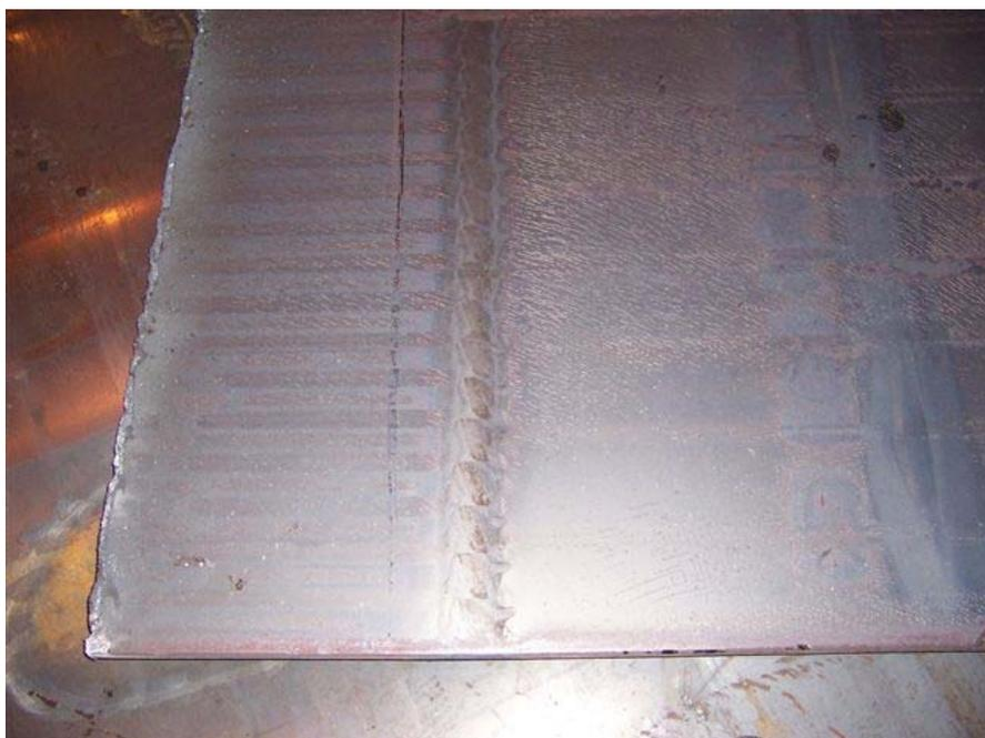
Figure 9 - Undescaled striping patterns on the surface due to non sufficient spray overlaps
