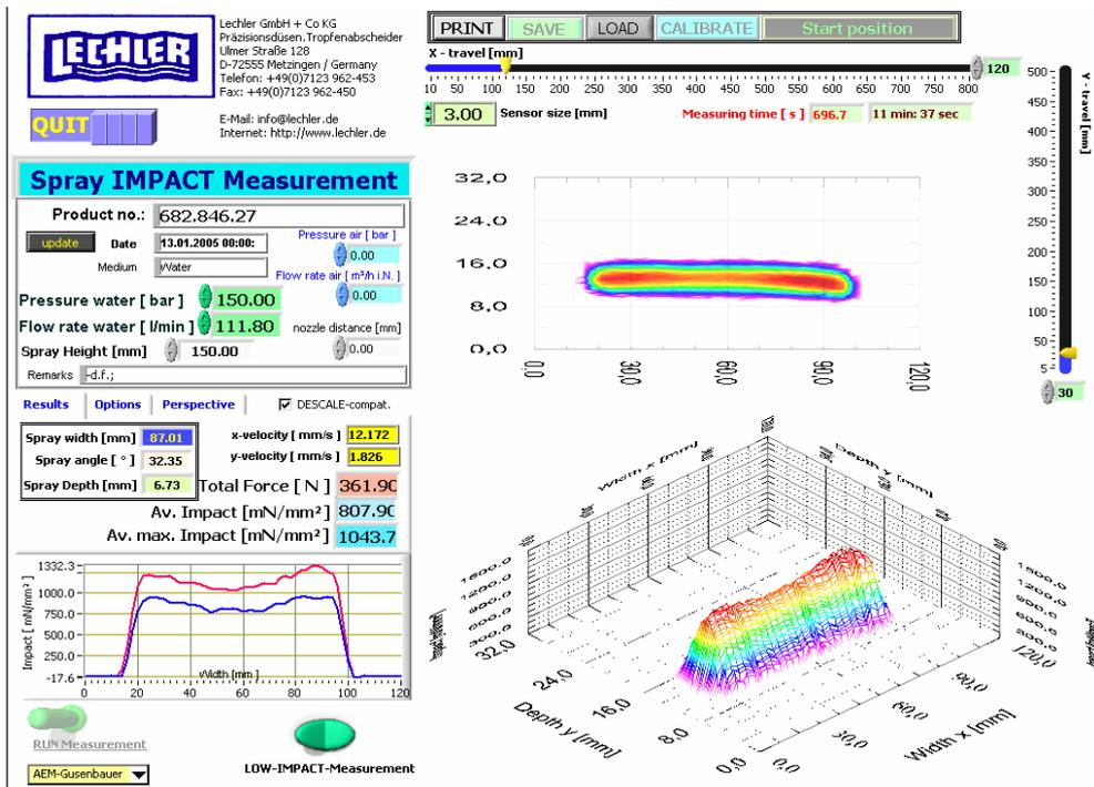
Figure 5 - Documented impact measurement of a descaling nozzle
