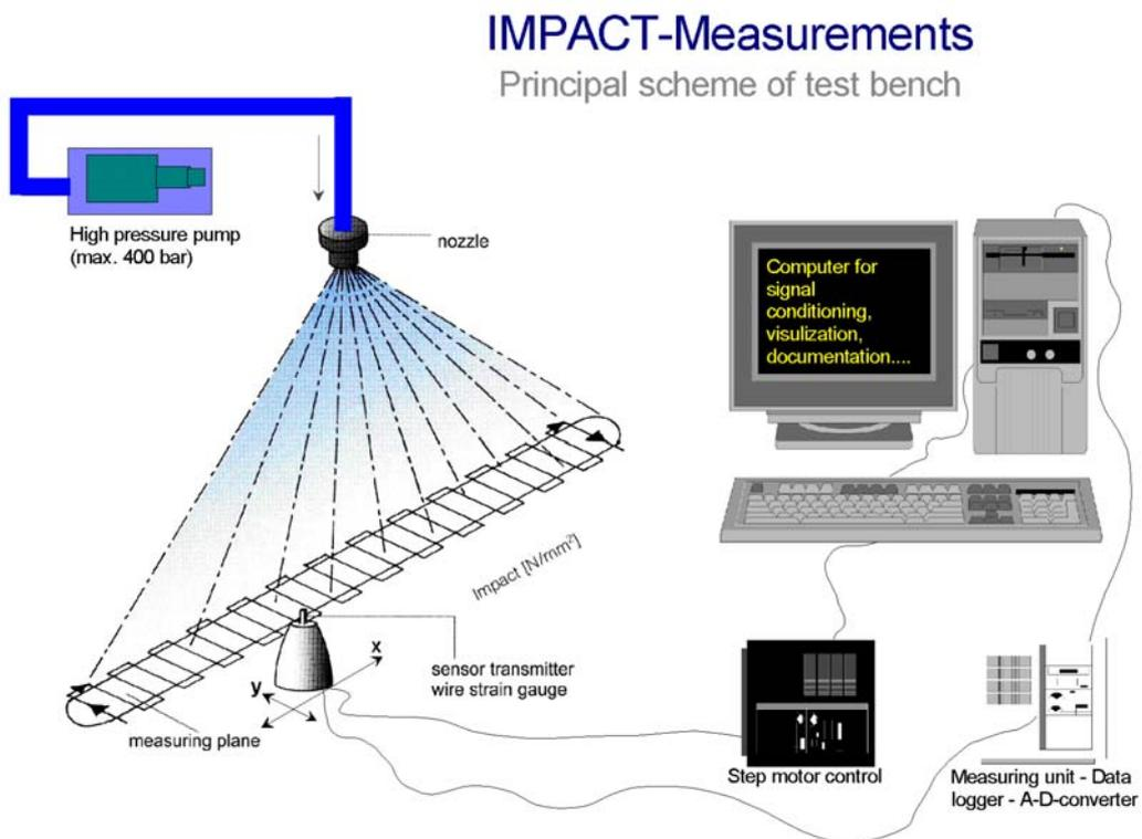
Figure 4 - Set-up of descaling nozzle in test bench for impact measurement.
