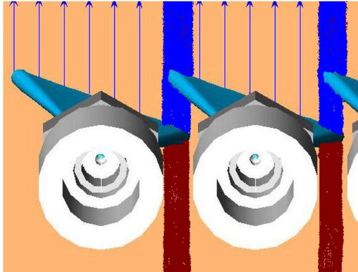
Figure 6 - Water layer effect caused by overlap being too big
