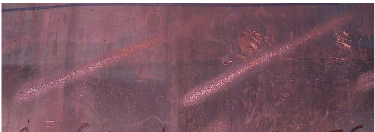
Figure 7 - No imprint on lead plate in the excessive overlap area
