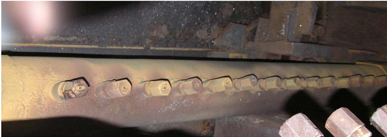
Figure 2 - Descaling header with poorly aligned nozzles
