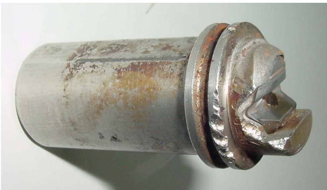
Figure 11 - Externally worn descaling nozzle tip caused by opposite header
