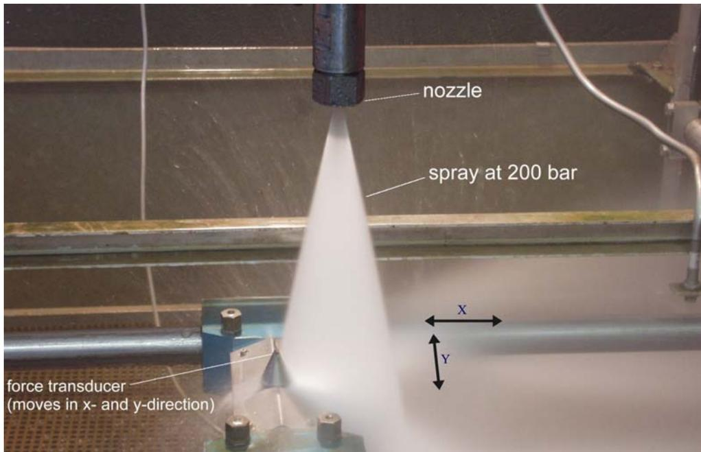
Figure 3 - Test bench to perform impact measurements
