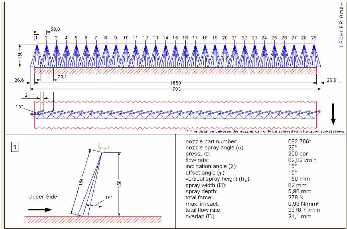
Figure 8 - Example of computer simulation with Lechler “DESCALE” program of existing situation with excessive overlap between adjacent sprays
