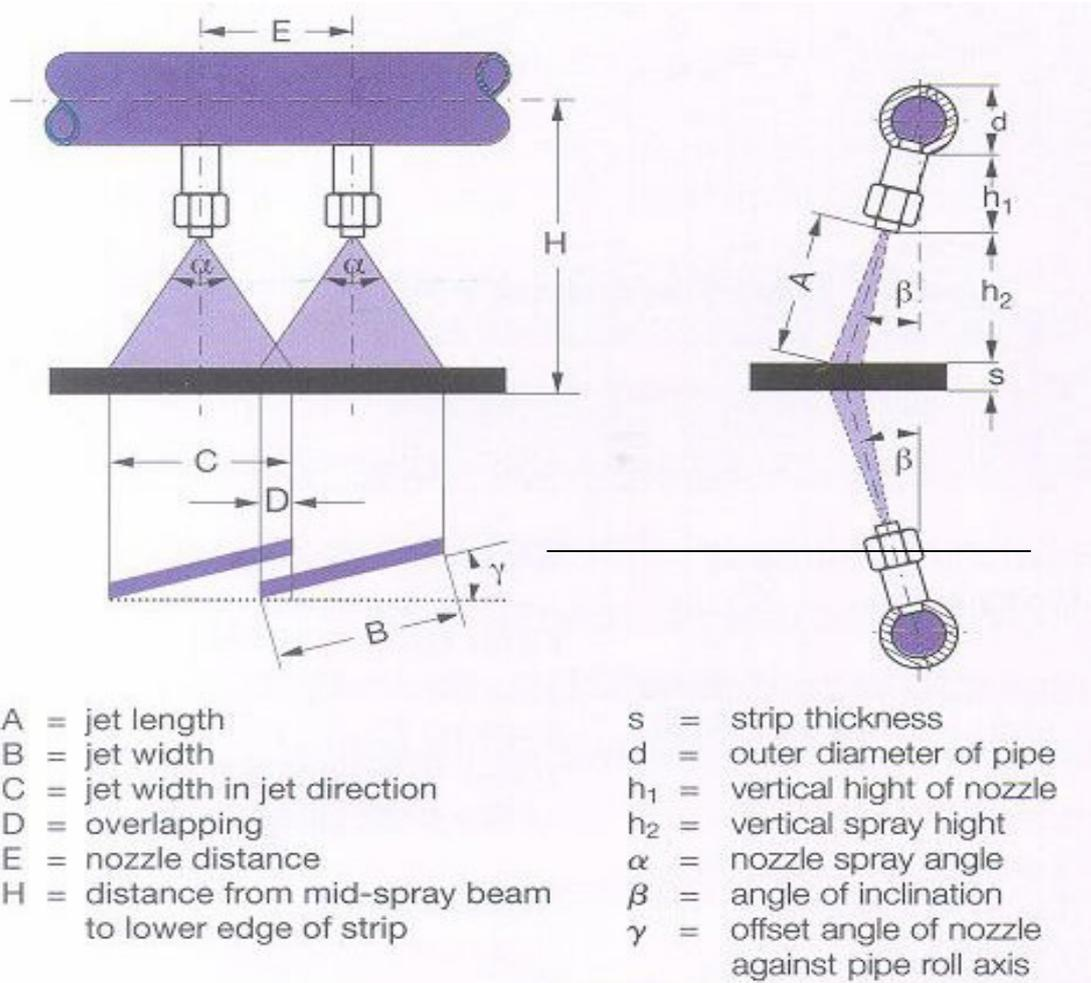
Fig.1: Nozzle arrangement with list of terms and symbols
