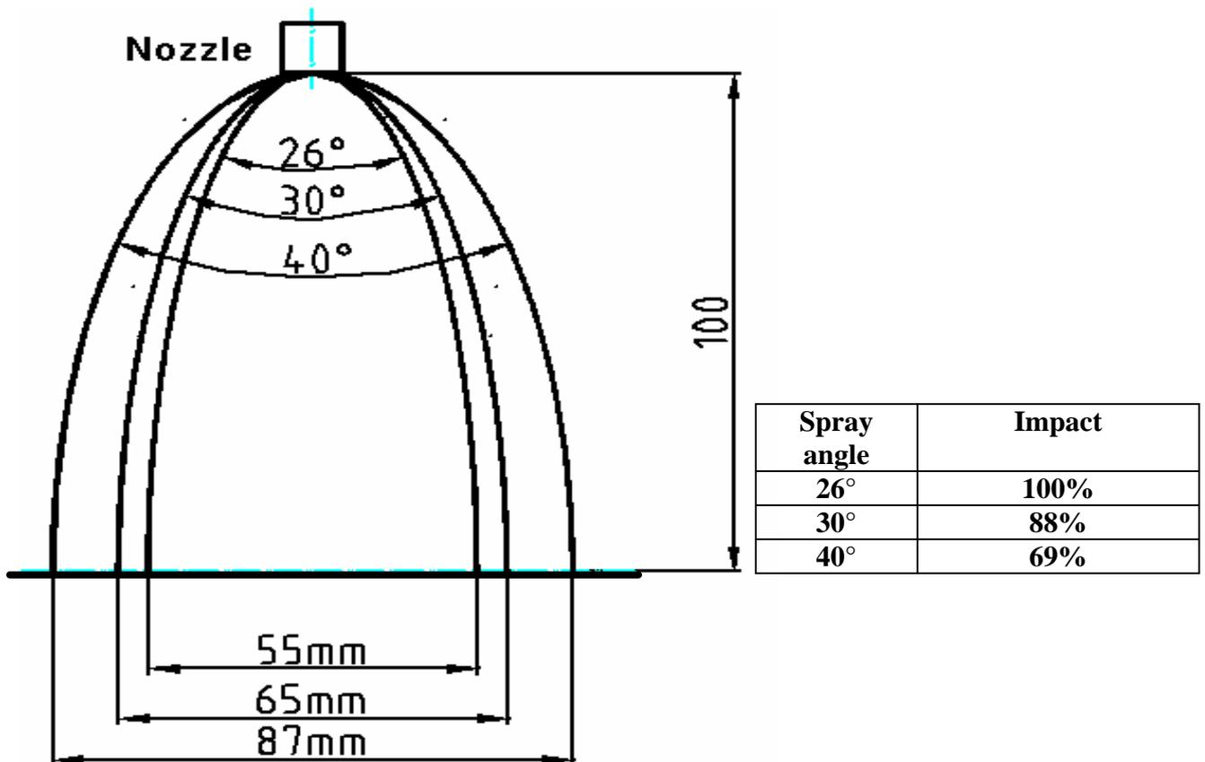
Fig. 8: Change of spray width and impact at different spray angles
