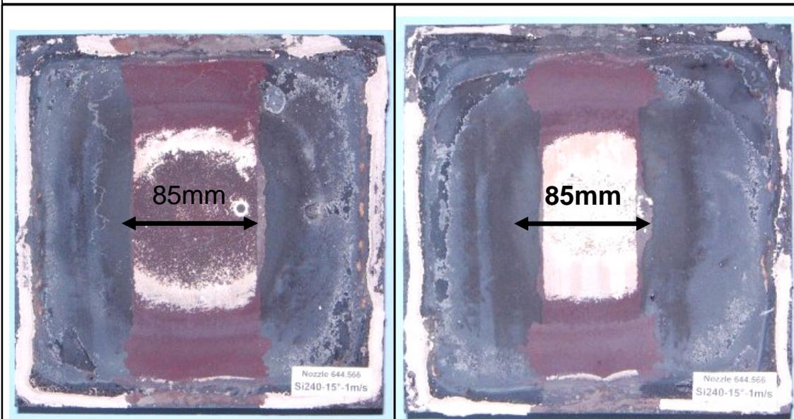
Fig. 5: Test plate, descaled at a spray height of 136mm. Remaining scale 24,9%
