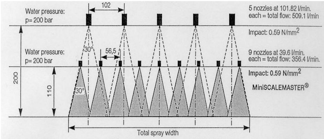
Fig. 7: Example of two nozzle arrangements at different spray heights with identical impact and significant reduction of water flow
