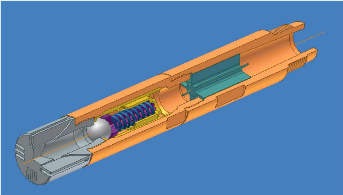
Fig. 11: Water Stop Valve WSV prevents undesired cooling of plates and strips
