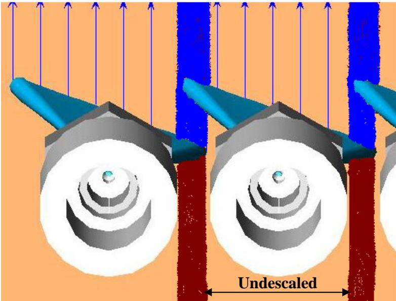
Fig. 9: Water layer effect caused by overlap being too big
