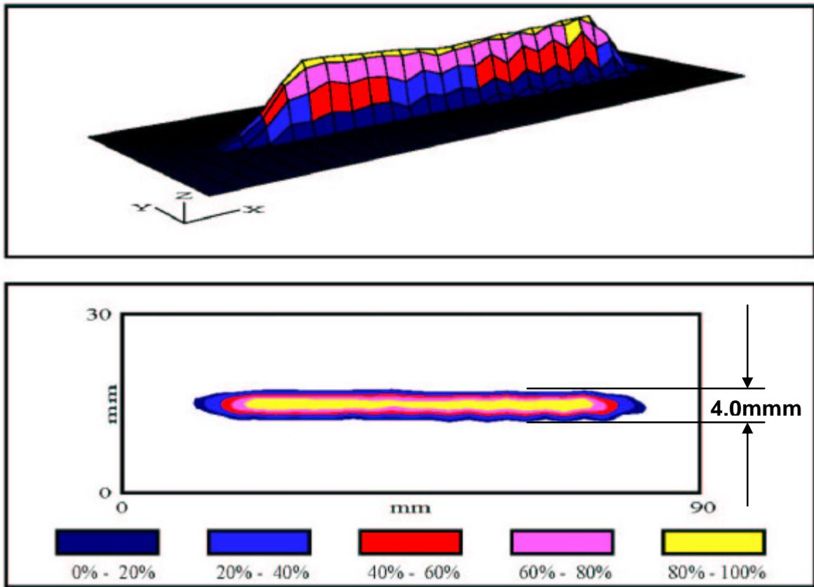
Fig. 2: Impact measurement of Scalemaster HP, 40° with 90 l/min at 400bar, max. impact 2,3N/mm at 80mm spray height, spray thickness 4,0mm
