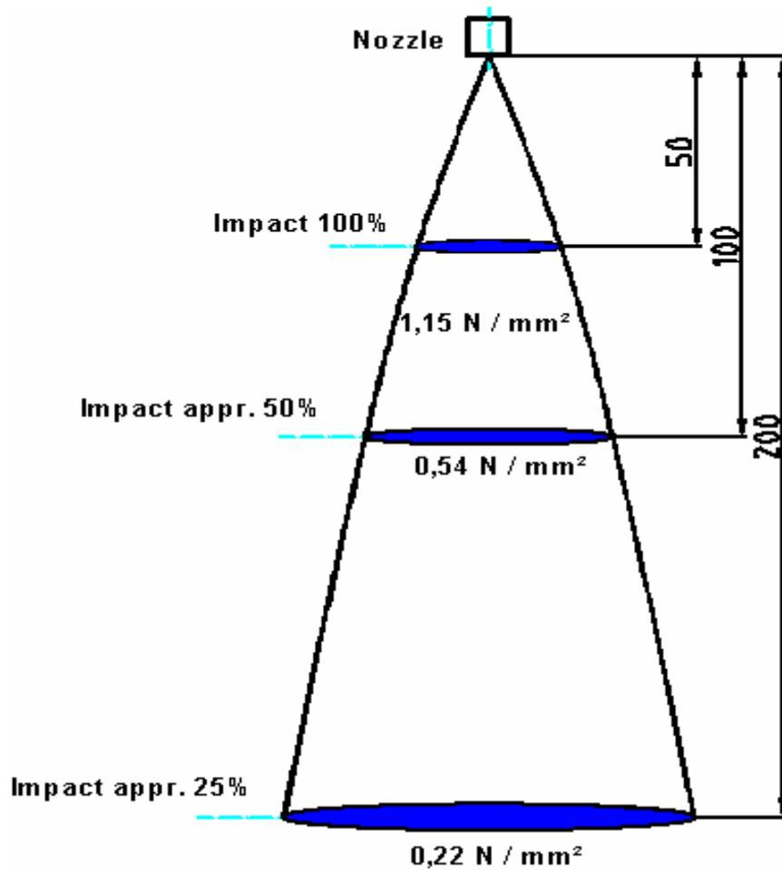
Fig.4: Effect of spray height on impact for a Standard Scalemaster with a flow of 25,5 l/min at 200bars and  $26^\circ$
