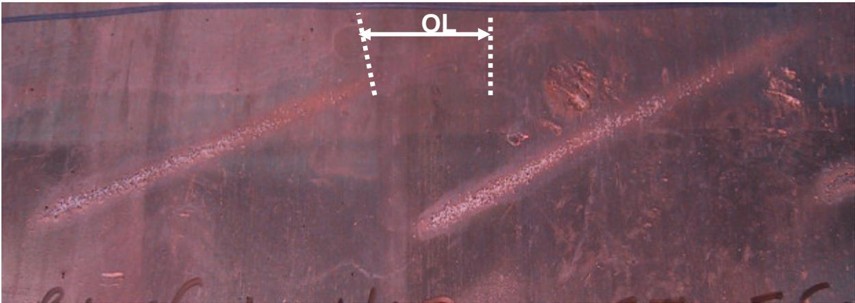
Fig.10: No imprint on lead plate in the excessive overlap area “OL”
